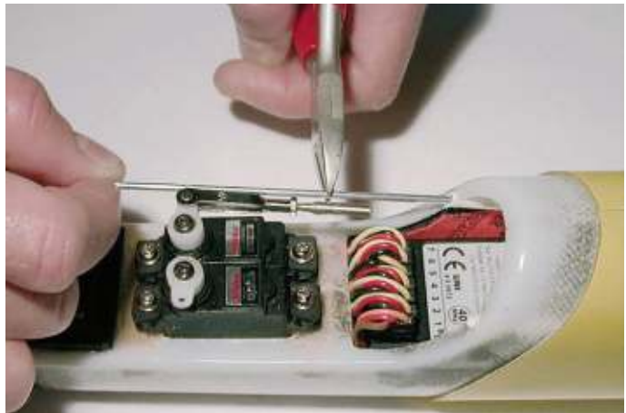
Fig.36: Shear the control rod.
