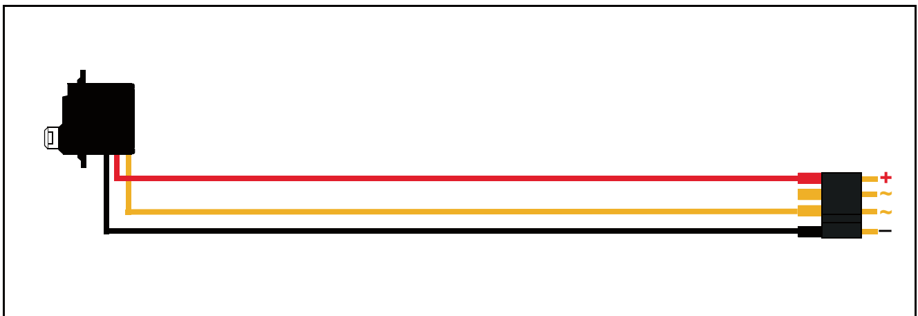
Fig.48: Servo soldered direct (aileron only version).
