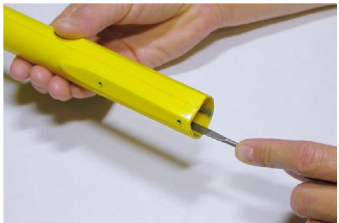
Fig.10: Remove the internal roughness.
