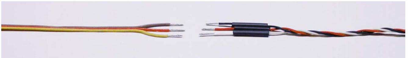
Fig.76: Wires ready for the soldering.
