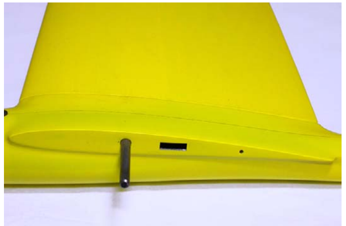
Fig.41: Insert a wing-panel.
