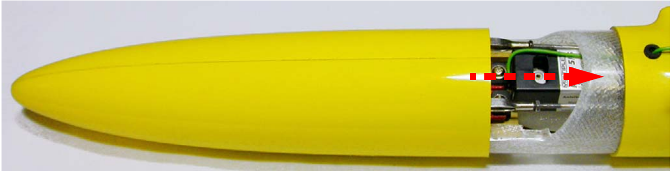
Fig.103: Installing the nose cone.
