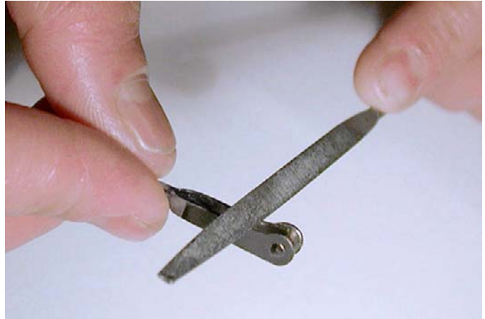
Fig.31: Remove part of the clevis.
