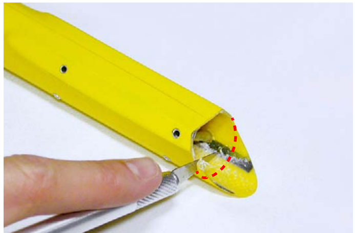
Fig.9: Remove the final part of the fuselage.
