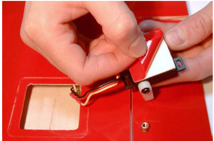
Fig.88:Apply the double adhesive plate.
