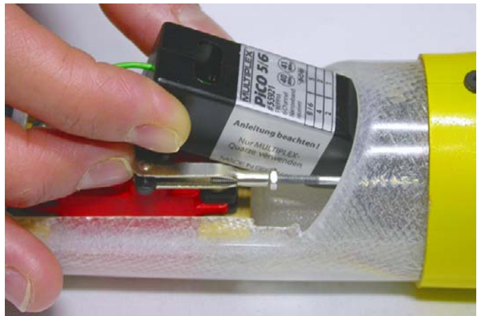
Fig.57: Positioning the receiver.
