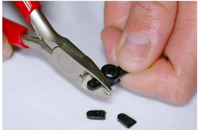
Fig.28: Cut the servo horns in surplus.
